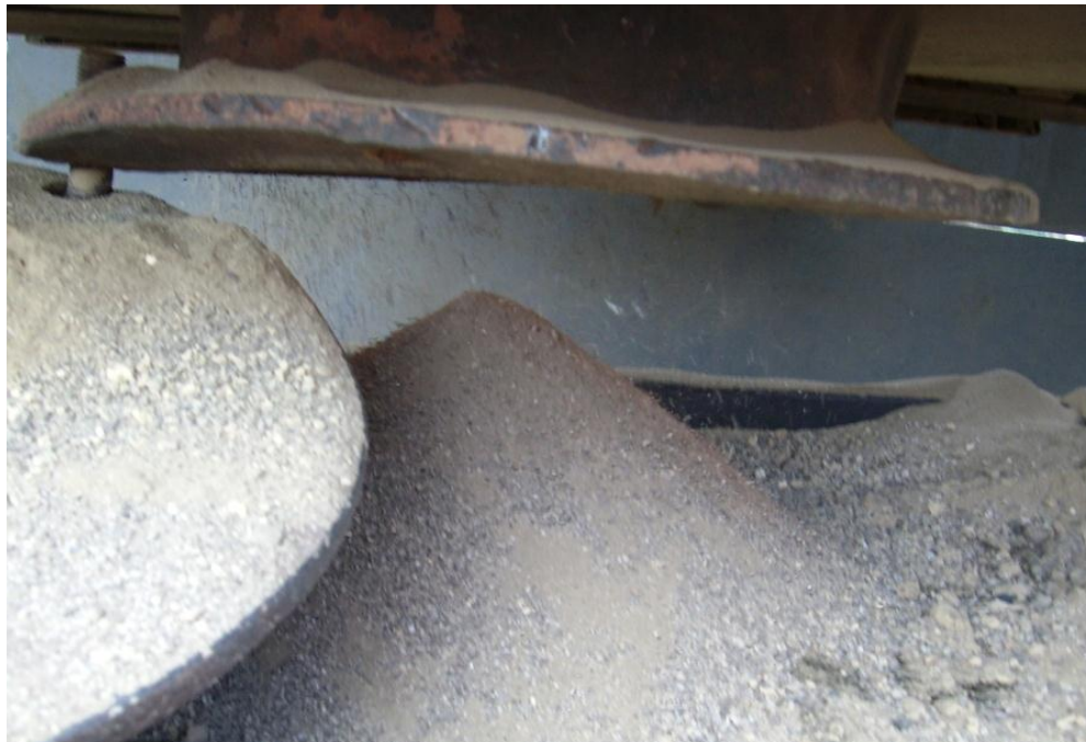
Coarse Ash from rotary kiln –Site Visit Feb 2012
